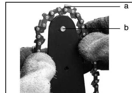
Hold the guide bar with the nose upwards and place the saw chain so on sprocket of the guide bar engage into the chain links and the bottom sections of the drive links are situated in the groove of the bar. The chain is correctly tensioned when it is still possible to raise it by 3-4 mm. The direction of rotation of the saw chain is indicated by two arrows on the drive-sprocket cover.
